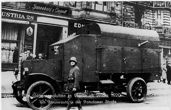
Two armored cars of improvised construction based on cargo transport chassis, being used by Freikorps troops. The combat value of such vehicles, which as a rule were fitted with untempered steel sheeting, remained low. Their existence stimulated the Reichswehr into creating armored wheeled vehicles; just as critical, though, was the analysis of operational experience. (WF)
