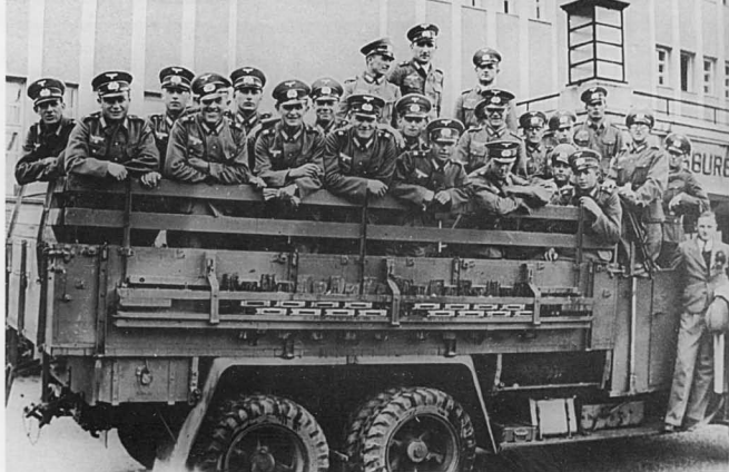
A large number of Henschel Typ 33 D1 6x4 medium all-terrain trucks were produced between 1933 and 1941. This photo was taken in the latter half of the 1930s. (MHM)
