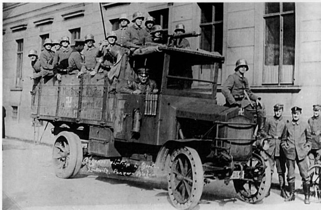
Berlin, March 1920. Troops of the Marinebrigade roll through the streets during the Kapp-Lüttwitz putsch. The front axle of this 3-ton Army transport is fitted with sprung steel wheels, a result of the acute shortage of rubber tires in Germany during the First World War which carried over into the postwar period. (WF)
