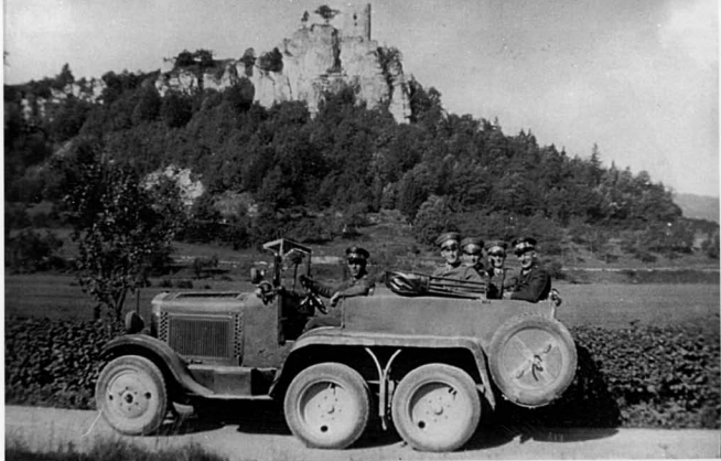
In 1926 the Reichswehr obtained a small quantity of six-wheeled all-terrain vehicles, including five Horch 8s. Gross weight was 4680 kg and an 8-cylinder Horch engine with 80 hp powered it, giving the vehicle a maximum speed of 70 kmh. (CK)
