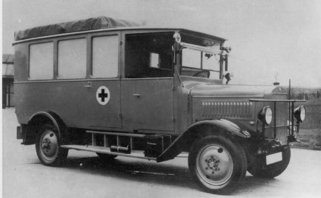
The Kfz. 31 ambulance. Characteristics of this vehicle, for which several types of commonly available cargo transports were used, were an enclosed body with windows, side and rear doors and luggage rack. The interior layout varied depending upon use. (WF)
