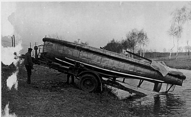
The Ah. 13 (trailer, single-axle) was used to carry motor boats by motorized and semi-motorized engineer bridge-laying units. It had an open frame design with equipment for loading and releasing a motorboat. (WF)
