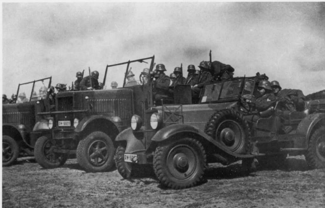
Above and below: The Wanderer W 11 was produced from 1933 on and acquitted itself well in operational use. 2844 vehicles were manufactured. These were used as command cars and in anti-tank companies of infantry regiments as tow vehicles for the 3.7 cm Pak L/45. (WF)
