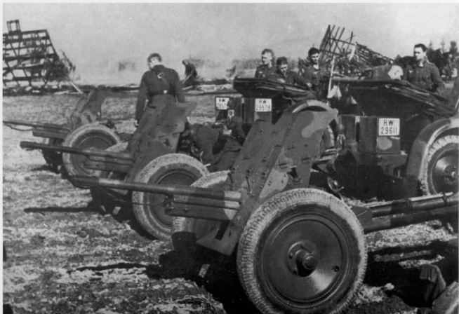
Above and below: The Wanderer W 11 was produced from 1933 on and acquitted itself well in operational use. 2844 vehicles were manufactured. These were used as command cars and in anti-tank companies of infantry regiments as tow vehicles for the 3.7 cm Pak L/45. (WF)
