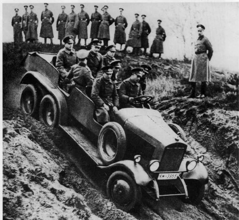
Right: Additional developments of the six-wheeled all-terrain vehicle were made by Daimler-Benz (in the form of the G 1 and G 3) and the Selve Automobilwerken AG in Hamelin. The G 3 shown in the picture was based on the 1.5-ton cargo transport chassis. (BA)
