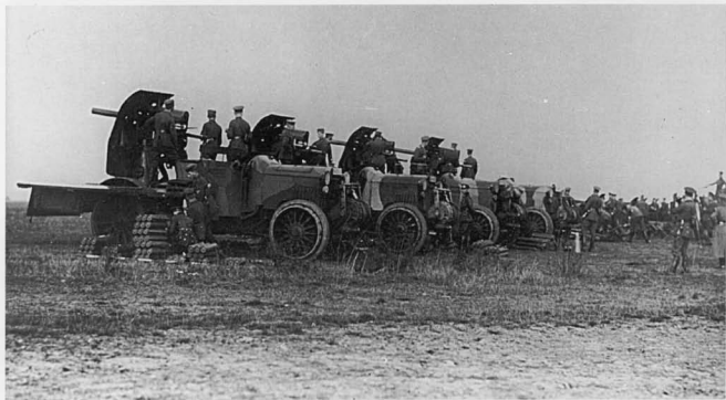
On the basis of a writ from the Wehramt of the Reichswehr, dated 25 March 1929, plans were made to refit the barrels of 120 anti-aircraft guns from 7.7 cm to 7.5 cm during the time period from 1930 to 1932. Of these, 80 were planned for the Kraftwagen 19 (Sd. Kfz. 1) gun platforms. Only 28 were permitted to be officially carried out. (CK)
