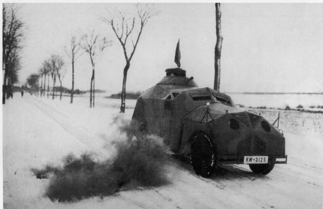
Above and below: Tank mockups based on personnel carrier chassis played a particularly important training role in the Reichswehr. Representative of the many, sometimes improvised tank dummies are the mockups shown here based on the Adler "Standard 6." They had a four-man crew and were produced from 1930 onward. (both BA)
