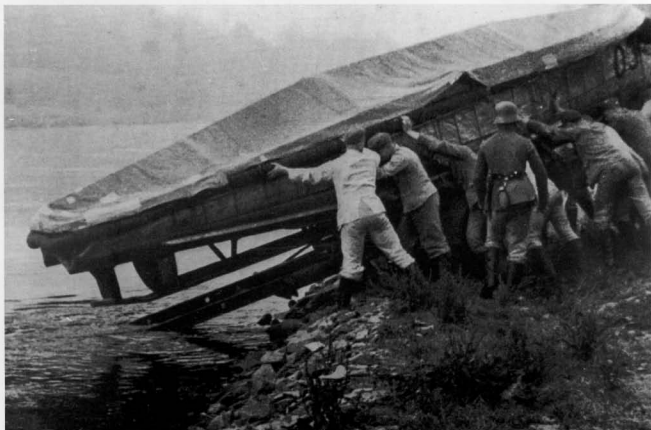
The Ah. 13 (trailer, single-axle) was used to carry motor boats by motorized and semi-motorized engineer bridge-laying units. It had an open frame design with equipment for loading and releasing a motorboat. (WF)
